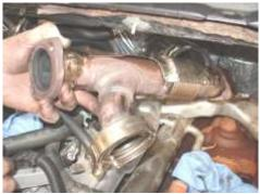
STEP 11: Loosen, the intake manifold bolts on the drivers side. Completely remove the intake manifold bolts on the passenger side and note their location with a piece of cardboard. Then remove the two bolts that go through the inner fan stator under the shroud.
