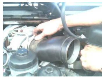
STEP 5: Continue by removing the charge pipe. Also unbolt alternator and disconnect wires. Tilt the alternator towards the front of the vehicle.
