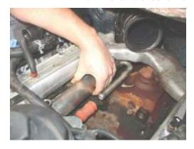
STEP 15: Install O-Rings on the SS EGR Cooler Bypass
