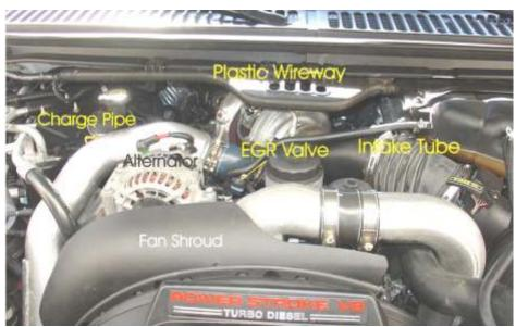
STEP 3: Pry the upper fan shroud away from the radiator and remove.
