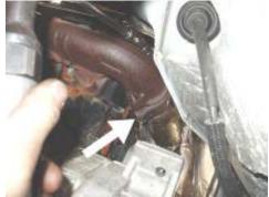
STEP 9: From the topside of the engine, loosen and remove bolts attaching the factory up-pipe to the y-pipe. Remove the y-pipe, giving you access to remove and replace the factory up-pipe.
