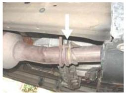
STEP 7: Remove turbo charger. This is done by removing the 2 oil feed line bolts, VGT actuator wire, Up-pipe v-band clamp, and the three turbo mounting bolts. Use penetrating oil on all turbo bolts, exhaust up pipe bolts, and pedestal bolts. Once these parts are removed, the turbo will roll toward the passenger side of the truck and out of the pedestal. Proceed to remove the pedestal as well as the oil drain tube from the H.P.O.P.
