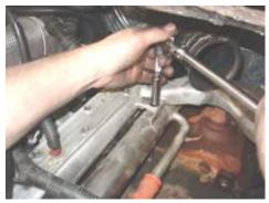
STEP 13: Lightly push down on the EGR cooler while pulling up on the intake manifold to disengage from the manifold.
