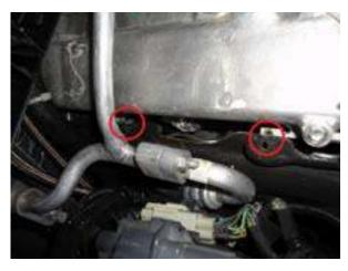
STEP 18: Remove the four 8mm bolts from the short EGR pipe and remove the short EGR pipe from vehicle. Retain bolts, gaskets and EGT sensor for later use.
