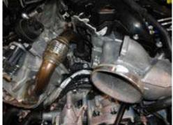
STEP 19: Remove the two 8mm bolts from the bracket holding the long EGR pipe to the EGR cooler. Remove the four remaining 8mm bolts from the long EGR pipe and remove the long EGR pipe from vehicle. Retain bolts and gaskets for later use.
