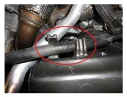
STEP 7: Disconnect clips and brackets holding the two larger coolant lines. Using pliers from the top of the vehicle, loosen the three factory clamps on larger coolant lines and pull lines off of connections.
