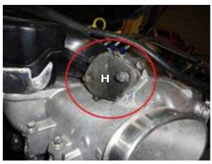
STEP 28: Slide the three supplied 8mm washers onto the three supplied 8mm bolts. Using the hardware, install the coolant block-off plate (largest plate). Tighten.
