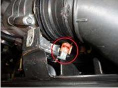
STEP 16: Remove 2 bolts holding wiring harness to front of EGR cooler.
