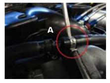
STEP 9: Using the factory clamp, install the short end of the coolant hose (L) on the coolant system reservoir. Route the hose (under the air box) towards the cold coolant system radiator. Slide over the nipple and tighten with provided hose clamps (D).
