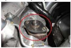
STEP 25: Unplug EGR outlet temp harness located under cast intake near the front of the engine. Remove ONE of the three EGT sensors from the factory exhaust and install it into the bung on the manifold block off plate and tighten.
