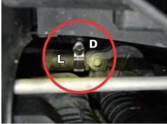
STEP 10: Disconnect the snap-fitted coolant line from the metal coolant pipe. Press tabs on both sides of fitting and slide off. Tuck line away from EGR system.
