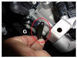
STEP 15: Unplug the EGR buterfly valve near the rad fan shroud.
