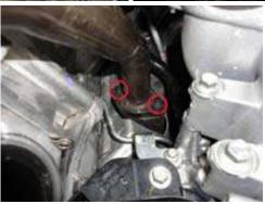
STEP 20: Remove the seven 8mm bolts holding the EGR system to the passenger side intake manifold. Remove the 10mm nut holding the pressure line bracket to the back side of the EGR cooler.
