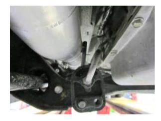
2.Installation of FLO-PRO system. Install pipe # 41711 with 4 hole flange by placing welded metal hanger into OEM transmission isolator as shown above. Loosely snug up 4 fasteners at downpipe (making sure that factory gasket is in place first). Install pipe # 41712 and # 41713, making sure to install hanger on 41713 into OEM isolator as shown below.
