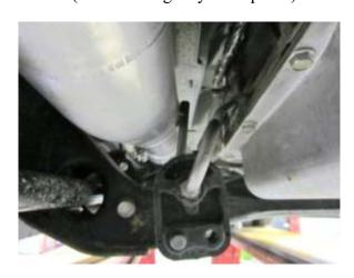
2. **Installation of FLO-PRO system.** Install pipe # 41711 with 4 hole flange by placing
