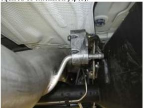
3. Install muffler delete # 90220, as well as over the axle pipe # 41115, placing metal hanger into OEM isolator.
