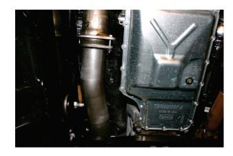
3. Next, install 61113NB pipe, 9454 extension pipe (Will need to be trimmed depending on wheelbase) and 7185 muffler.
