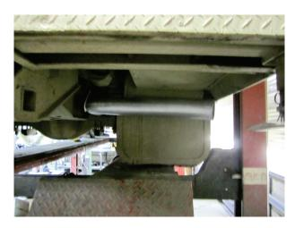
5. With the pipes mounted loosely, adjust the new Flo-Pro system for clearance and appearance. Evenly tighten all clamps starting with the front flange connection working your way to the back.
