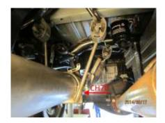
4. With the pipes mounted loosely, adjust the new Flo-Pro system for clearance and appearance. Evenly tighten all connections and clamps starting with the front flange connection working your way to the back.
