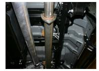
4. With the pipes mounted loosely, adjust the new Flo-Pro system for clearance and appearance. Evenly tighten all clamps starting with the front flange connection working your way to the back.
