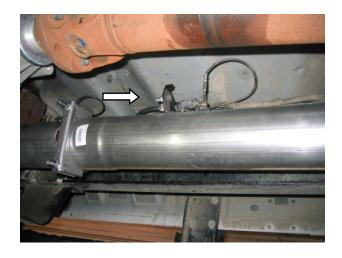
3. Install muffler replacement pipe by placing clamp hanger supplied over the inlet of muffler and place into OE rubber hanger.
