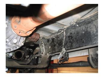
2. Install pipe with flange by placing welded metal hanger into OE rubber hanger and loosely tighten flanges together. Install 60813 pipe with the pre-welded bracket pointing upwards. Place the clamp hanger supplied into the OE rubber hanger. Install extension pipes depending on wheelbase. Install line/sensors from diesel particulate filter back onto the new system.
