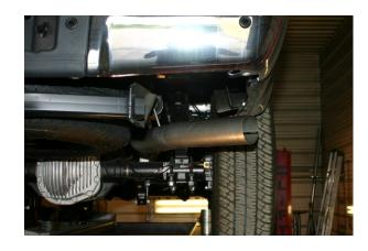
6. With the pipes mounted loosely, adjust the new Flo-Pro system for clearance and appearance. Evenly tighten all clamps starting with the front flange connection working your way to the back.
