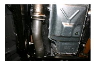
3. Next, install 61113NB pipe, extension pipe (for Crew Cab Long Box) and Y-pipe. You can use a stand to support the Y-pipe in place.
