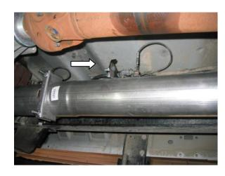
3. Install Ypipe by placing clamp hanger supplied over the inlet of Ypipe.
