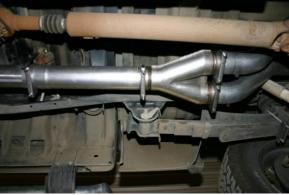
4. Install the driver's side exhaust pipe into left outlet of "Y" pipe. Place the metal hanger into the OE rubber hanger. Install the left tail pipe onto the outlet of left exhaust pipe and place strap hanger to frame using the second hole from end and rubber should be under frame when complete, tighten bolt in strap hanger completely. Install clamps on left connections.
