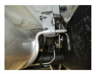
3. Install muffler delete # 95220, as well as over the axle pipe # 41156, placing metal hanger into OEM isolator.
