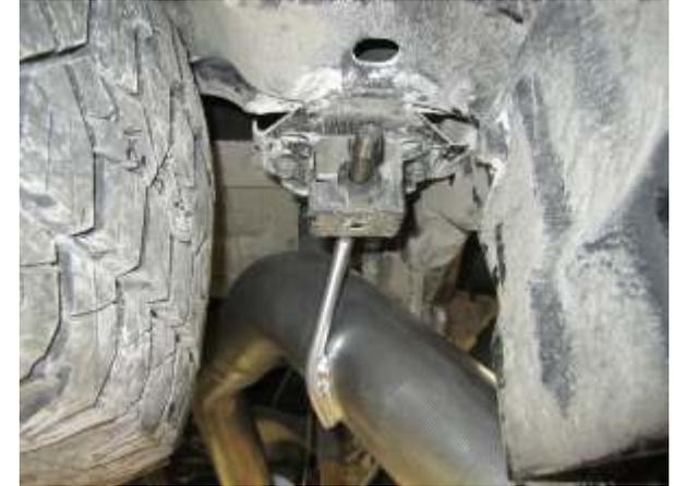
6. With the pipes mounted loosely, adjust the new Flo-Pro system for clearance and appearance. Evenly tighten all clamps starting with the front flange connection working your way to the back.
