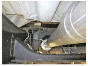
3. Install muffler delete # 40220, as well as over the axle pipe # 11725, placing metal hanger into OEM isolator.
