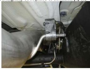
3. Install muffler delete # 40220, as well as over the axle pipe # 11115, placing metal hanger into OEM isolator.
