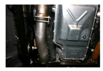
3. Next, install 31113NB pipe, extension pipe (for Crew Cab Long Box) and muffler delete.
