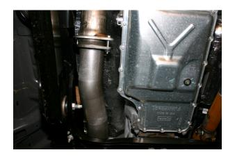
3. Next, install 31113NB pipe, extension pipe (for Crew Cab Long Box) and muffler. You can use a stand to support the muffler in place.
