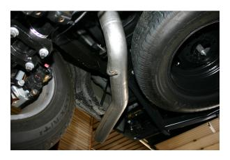
5. With the pipes mounted loosely, adjust the new Flo-Pro system for clearance and appearance. Evenly tighten all clamps starting with the front flange connection working your way to the back.
