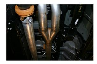
4. Install driver's side over-the-axle pipe into left outlet of "Y" pipe. Place the metal hanger into the OE rubber hanger. Mount the supplied strap hanger onto the frame (see picture) and then install the driver's side tail pipe, placing metal hanger into the strap hanger.
