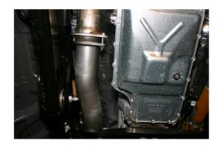
3. Next, install 31113NB pipe, extension pipe (for Crew Cab Long Box) and Y-pipe. You can use a stand to support the Y-pipe in place.
