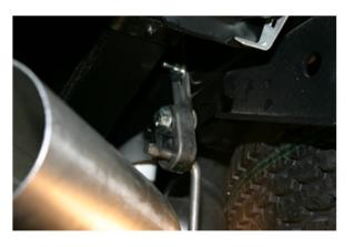
5. Install the right over-the-axle exhaust pipe into right outlet of "Y" pipe, placing metal hanger into OEM rubber mount. Then install the right tail pipe, placing metal hanger into OE rubber hanger.
