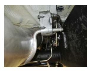
3. Install muffler as well as over the axle pipe # 11156, placing metal hanger into OEM isolator.
