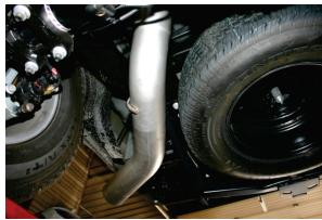
5. With the pipes mounted loosely, adjust the new Flo-Pro system for clearance and appearance. Evenly tighten all clamps starting with the front flange connection working your way to the back.
